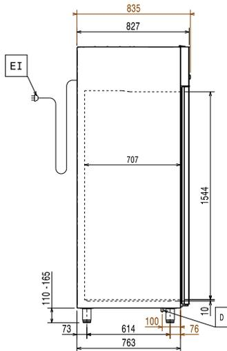
ED = Remote electrical connection      RO = Refrigerant Outlet
